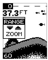
This is the zoom size menu. Zoom size is the distance between the upper limit and the lower limit. The upper limit shows at the top left corner of the screen. The lower limit is in the bottom left corner. For example, if the upper limit is 40 feet and the lower limit is 70 feet, the zoom window size is 30 feet. The word "TRACK" appears in this menu when you first activate the zoom as shown below. This means the X-45 is tracking the bottom in a zoom window, always keeping it on the display.
